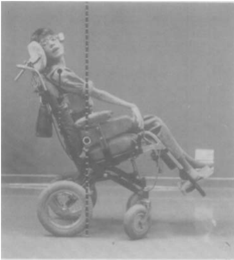
Fig. 3. Sitting in original position, in own adapted 'Relax' chair. Line of gravity (arrow) is posterior to fulcrum at ischial tuberosities (circle). Postural control and arm and hand function were worst on this position and pathological movements (asymmetric tonic neck reflex) were most frequent.
